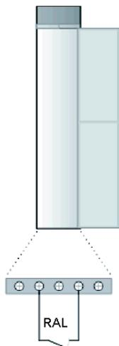
When your Hot Standby system is operating normally, with the PLCs in either the Run Primary or Run Standby operating modes ([see page 33](#)), the alarm relay is activated and its contact is closed (state 1). Whenever one of your PLCs enters the Stop or Offline operating modes, or when the power supply drops out or loses its supply power, the alarm relay falls back and its associated relay opens (state 0). This figure illustrates these behaviors:
