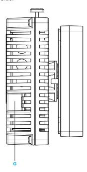
**G** Mini-B USB port connector: connects the data transfer PC cable to the unit.
