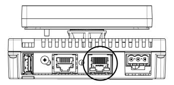
Do not confuse the RJ45 Ethernet connector with the RJ45 COM1/COM2 serial port.
